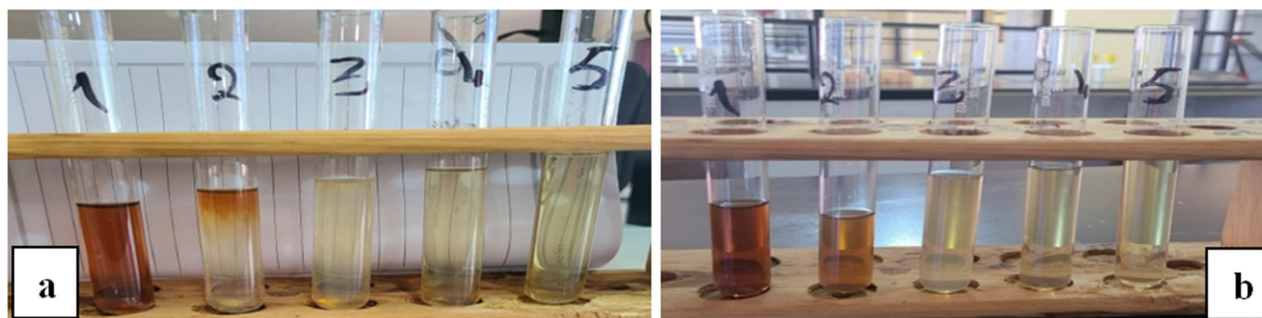
Figure 1. Colour change in five concentrations of P. guajava with silver solution. (a): Initially after adding extract to silver solution; (b): After 45 minutes from adding extract to silver solution.
